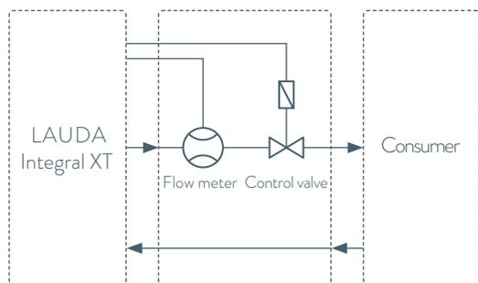
Through-flow control range: 0.2 ... 20 L/min
